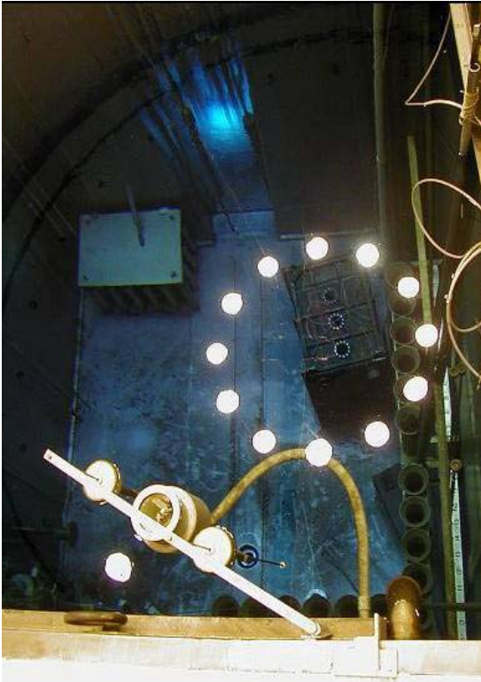
Figure C-2. TAMU NSC Reactor Pool with Reactor Under Power. This picture shows the large TAMU NSC reactor pool with the reactor located in the “stall” position at the top of the photo. The cross sectional schematic shows the pool, stall, dry irradiation cell, and 5 beam port locations. Also pictured in the upper left of the photograph is the spent fuel from the original NSC core (in the large “box-shaped” object to the lower left of the reactor).
