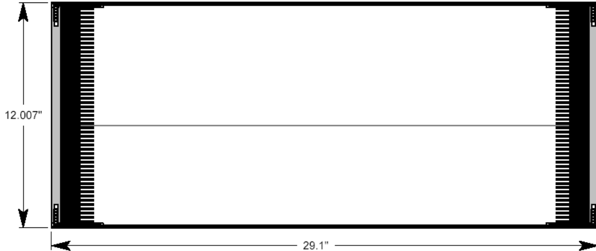
Figure A-2. Top view of an aluminum fuel tray. The dimensions in this drawing are 30.7 cm x 73.9 x 8.1 cm high (12 in x 29.1 in x 3.2 in high). While the length and height of the final trays will remain, the width will depend on the final configuration of the core and optimum placement and spacing for the fuel plates. Widths for the six trays may vary between 10 and 20 cm (4 and 8 inches). A single fuel plate is also illustrated.
