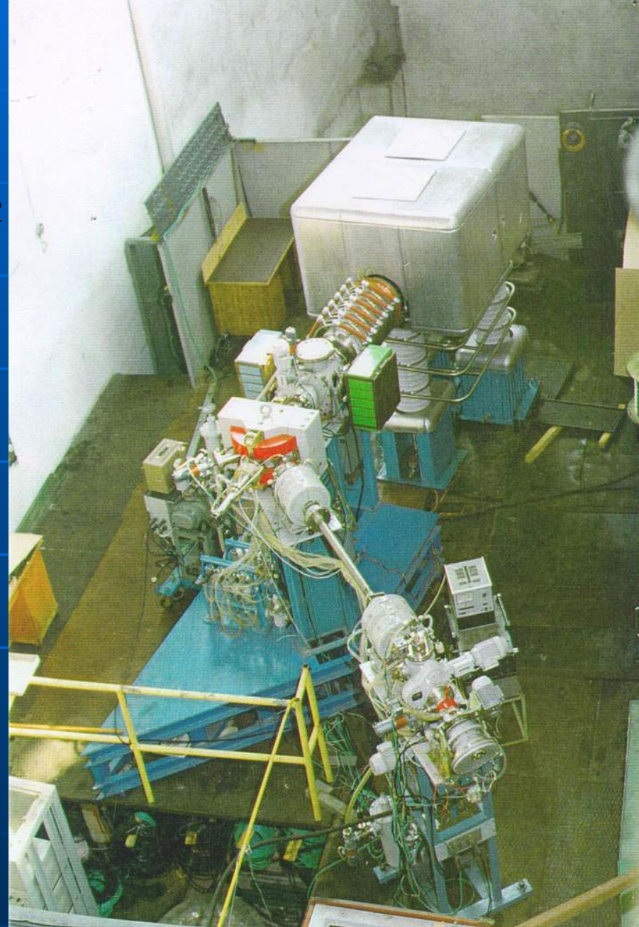
Neutron generator NG-12-1 ( D+^3H \rightarrow n+^4He ; D+D \rightarrow n+^3He )
