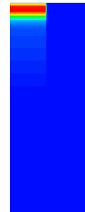
CAST3M Power Density Distribution for a 1 kW Beam Power
