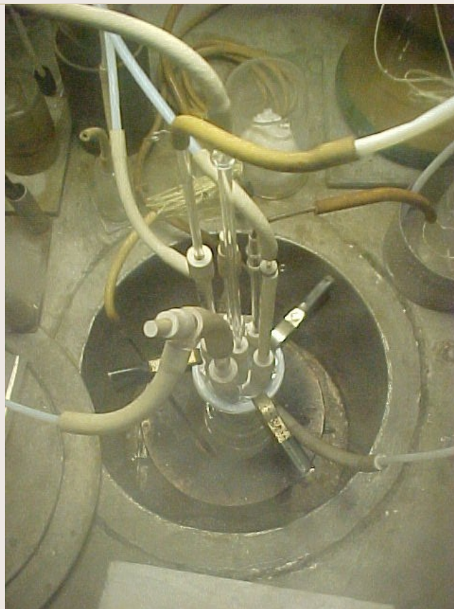
Electrochemical cell for oxide barium titration
