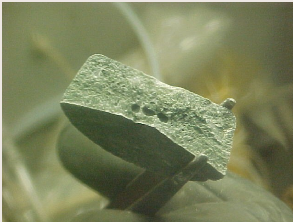
Fragment of the NaCl-2CsCl + 3wt% CmCl 3 salt ingot
