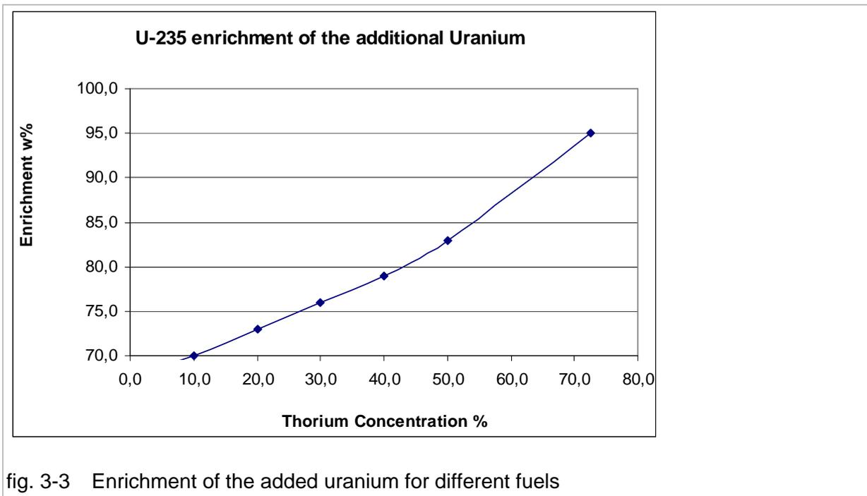
fig. 3-3 Enrichment of the added uranium for different fuels
