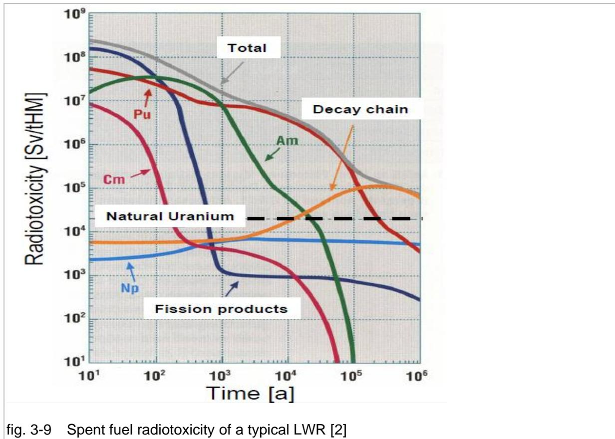
fig. 3-9 Spent fuel radiotoxicity of a typical LWR [2]
