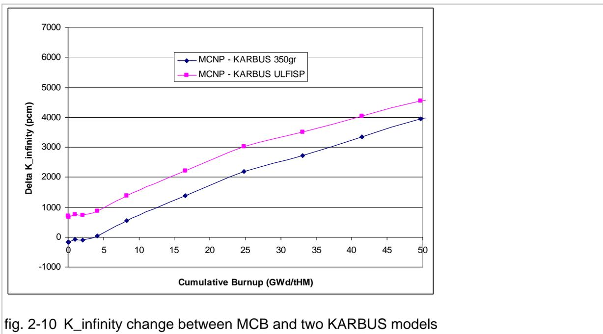
fig. 2-10 K\_infinity change between MCB and two KARBUS models
