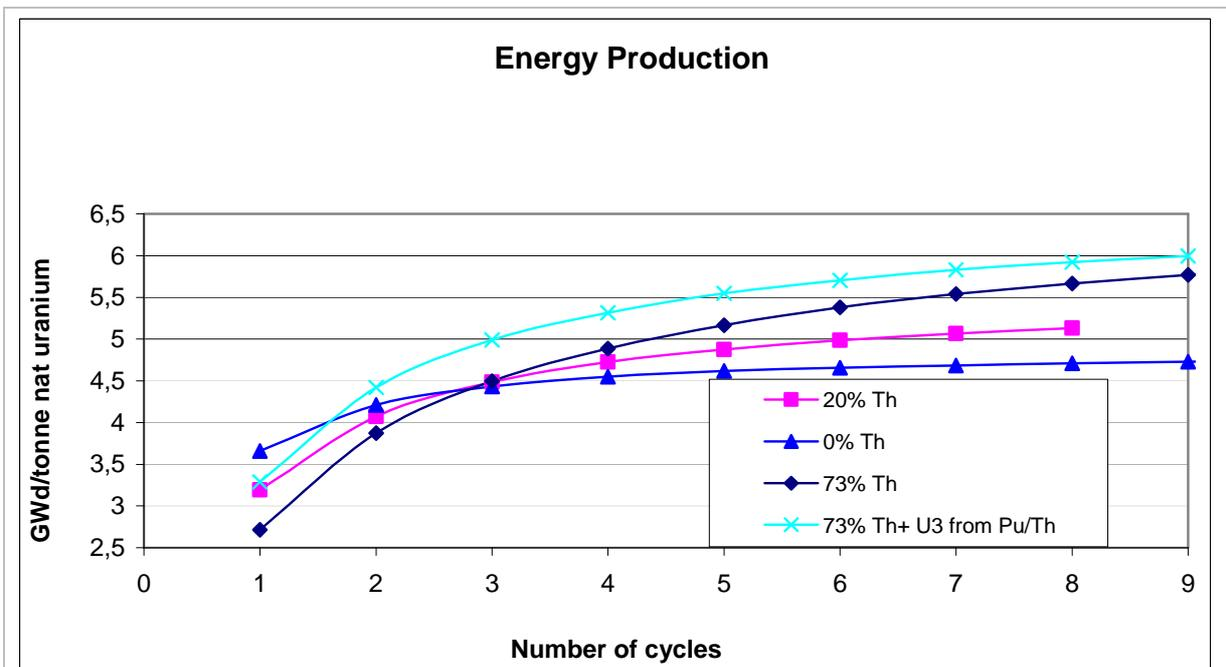
fig. 4-7 Energy production per unit of Natural Uranium consumed after each recycling for different fuels
