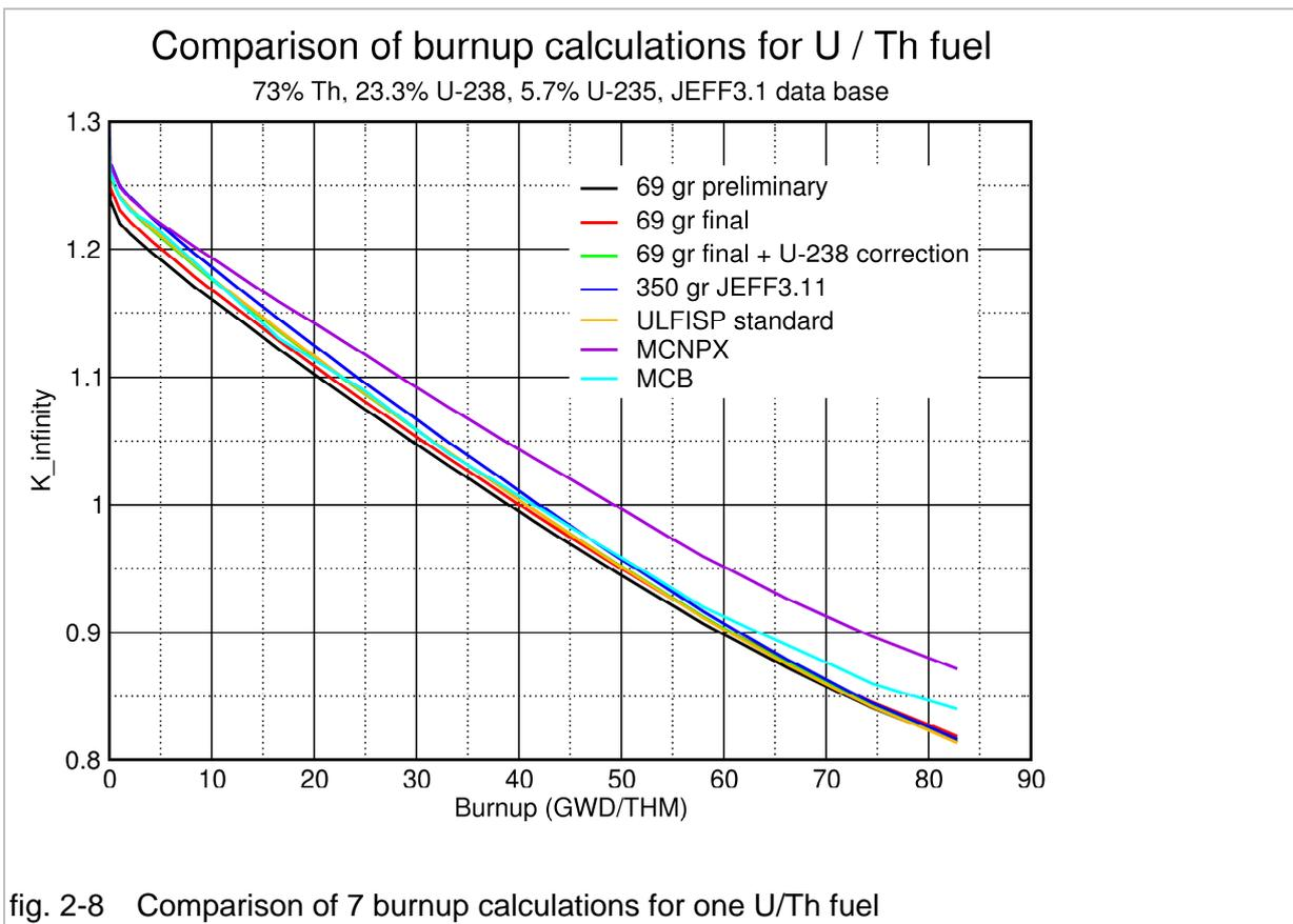
fig. 2-8 Comparison of 7 burnup calculations for one U/Th fuel
