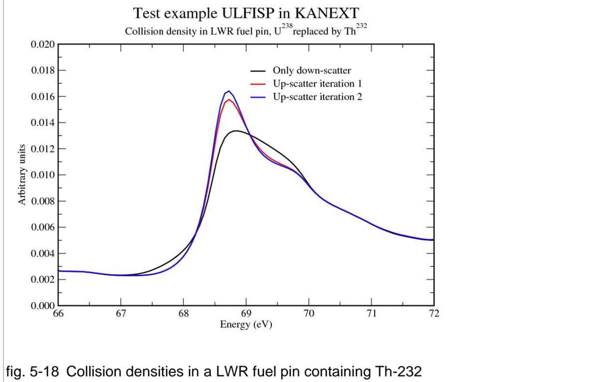
fig. 5-18 Collision densities in a LWR fuel pin containing Th-232
