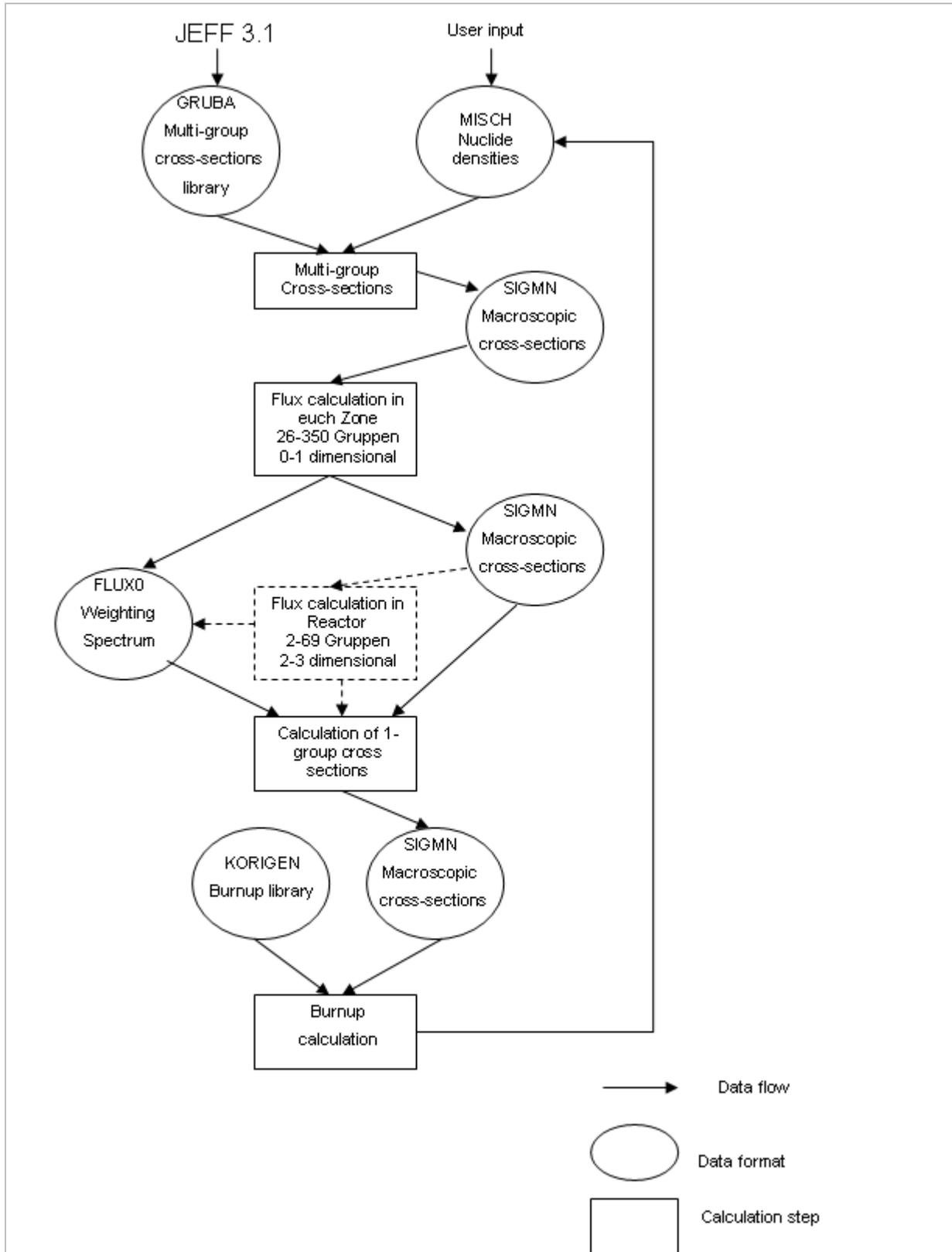
fig. 2-7 KARBUS calculation procedure [7]
