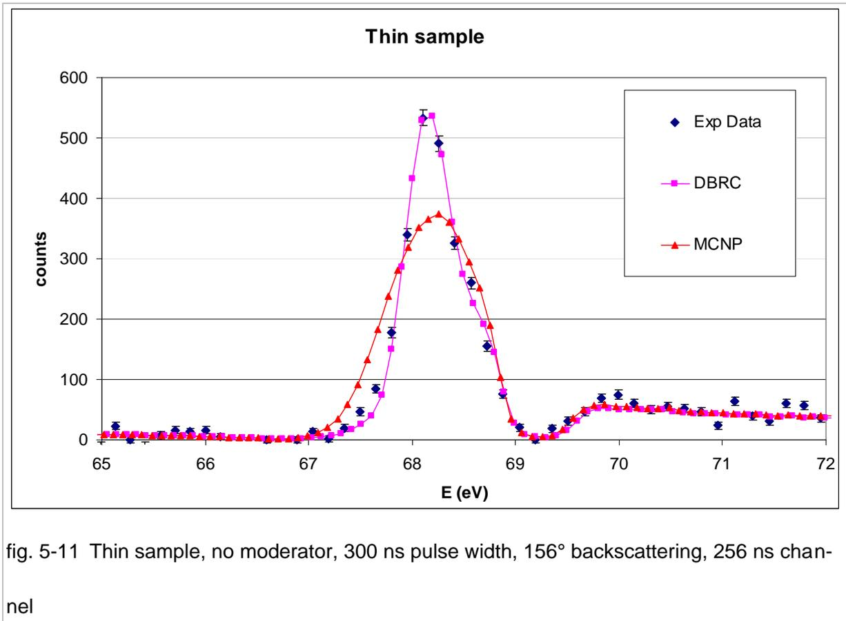
fig. 5-11 Thin sample, no moderator, 300 ns pulse width, 156° backscattering, 256 ns channel
