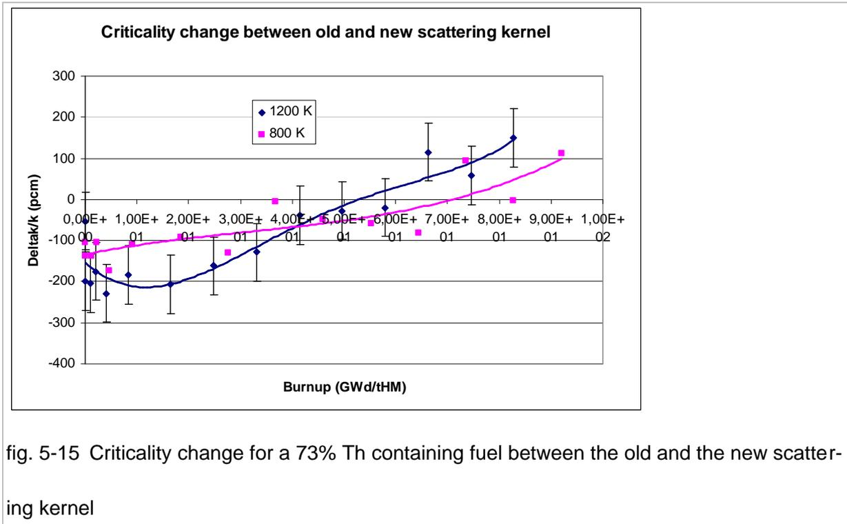
fig. 5-15 Criticality change for a 73% Th containing fuel between the old and the new scattering kernel
