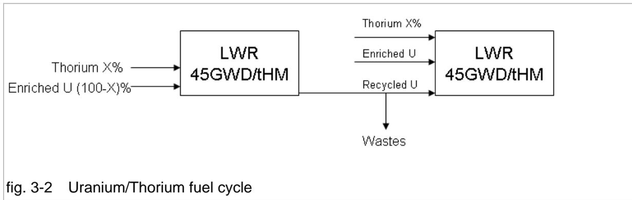
fig. 3-2 Uranium/Thorium fuel cycle
