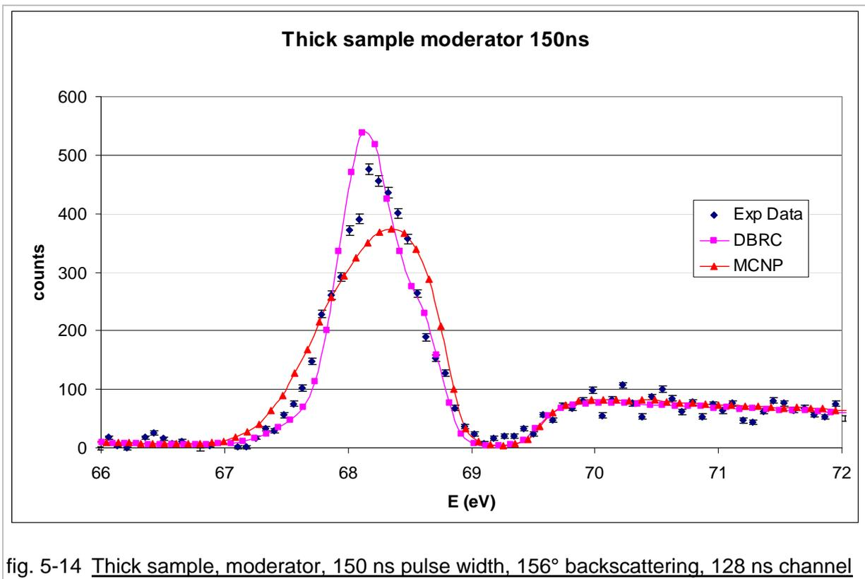
fig. 5-14 Thick sample, moderator, 150 ns pulse width, 156° backscattering, 128 ns channel
