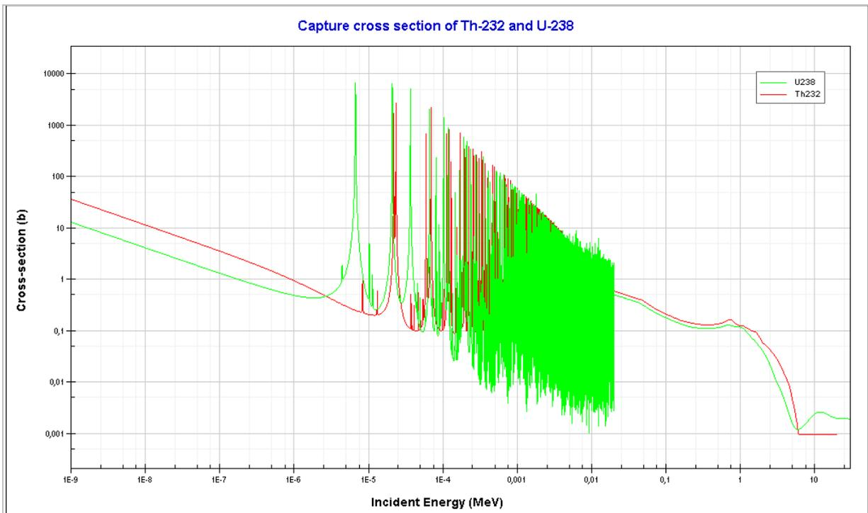
fig. 1-3 Capture Cross Section of Th-232 and U-238
