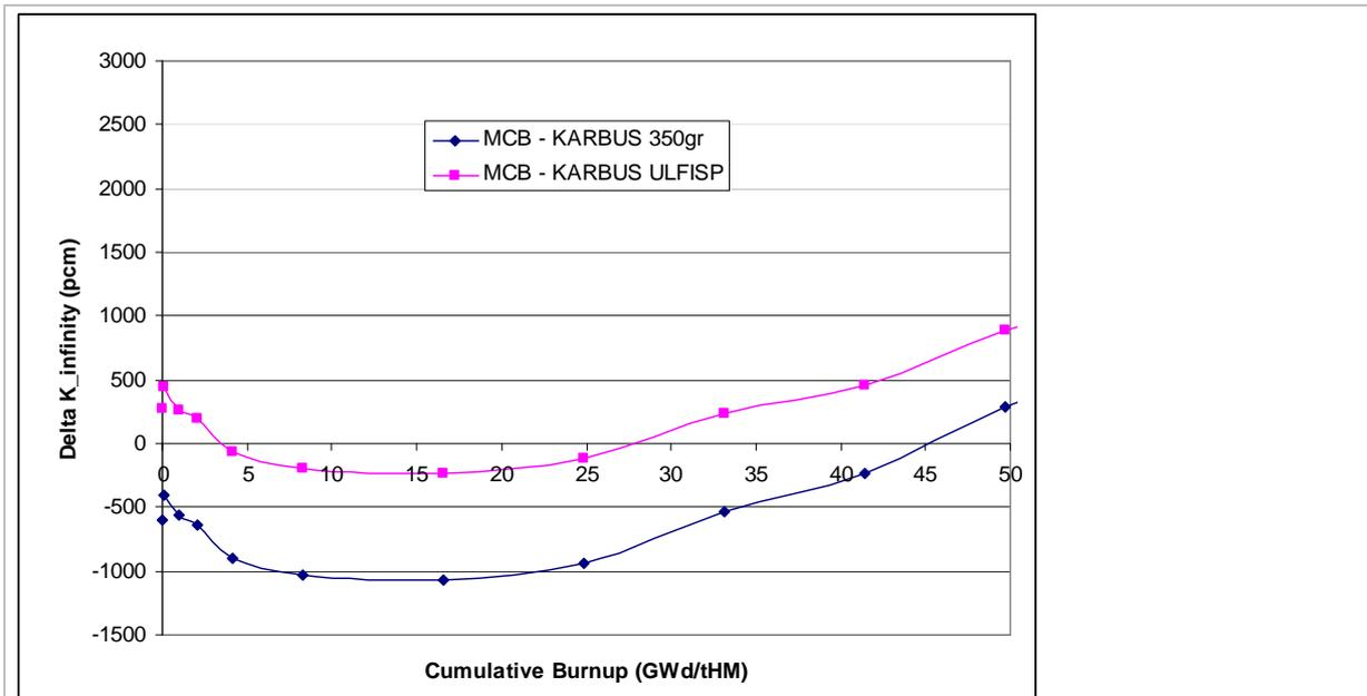
fig. 2-9 K\_infinity change between MCB and two KARBUS models
