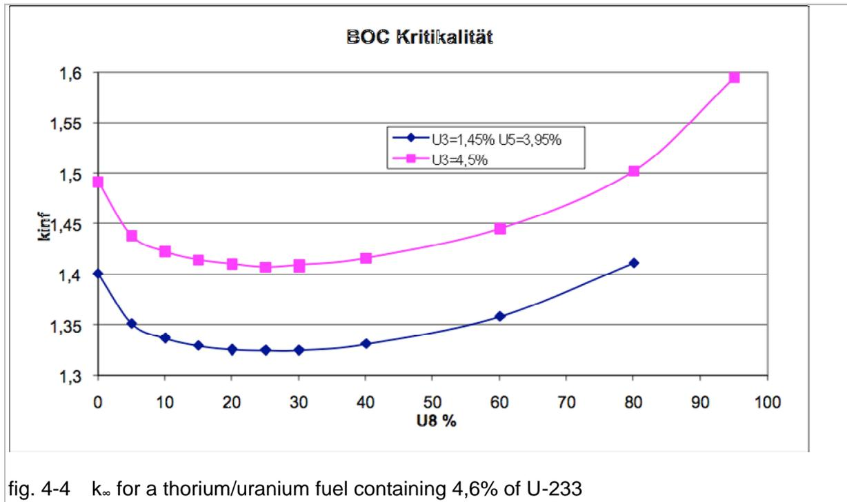
fig. 4-4  $k_{\infty}$  for a thorium/uranium fuel containing 4,6% of U-233
