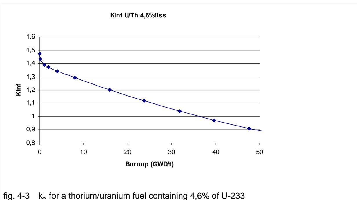
fig. 4-3  $k_{\infty}$  for a thorium/uranium fuel containing 4,6% of U-233
