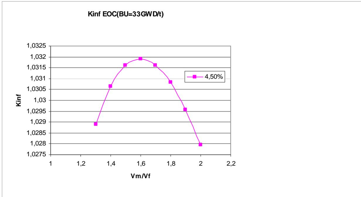
fig. 4-2  $K_{infinity}$  at the EOC for different moderation ratios
