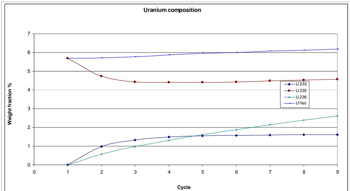
fig. 3-5 Uranium composition along the cycles for a 73% Th fuel at the BOC
