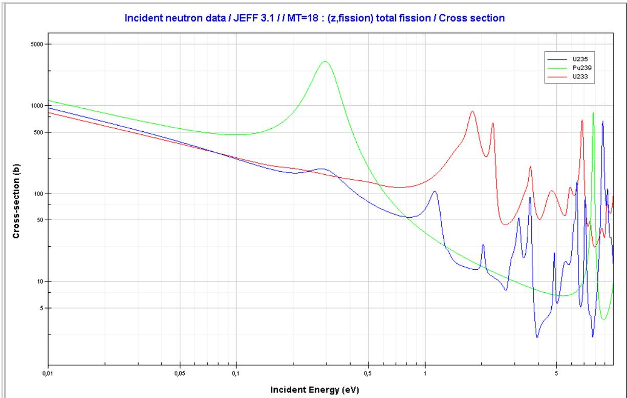
fig. 1-4 Fission cross-section of U-233, U-235 and Pu-239
