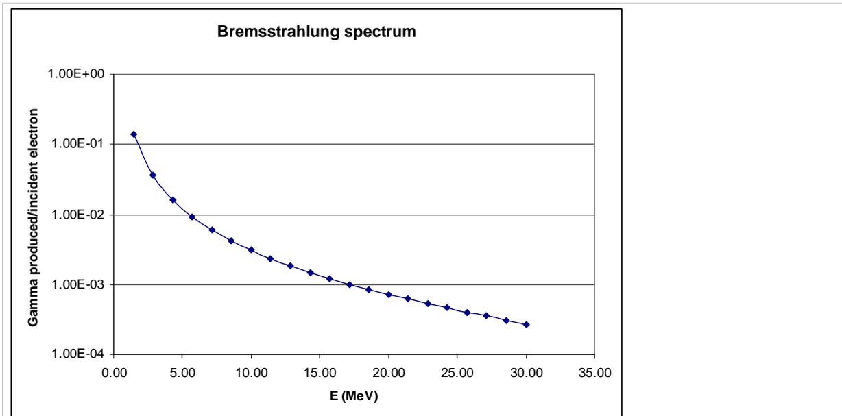
fig. 5-6 Bremsstrahlung spectrum of the Tantalum simulated with MCNPX
