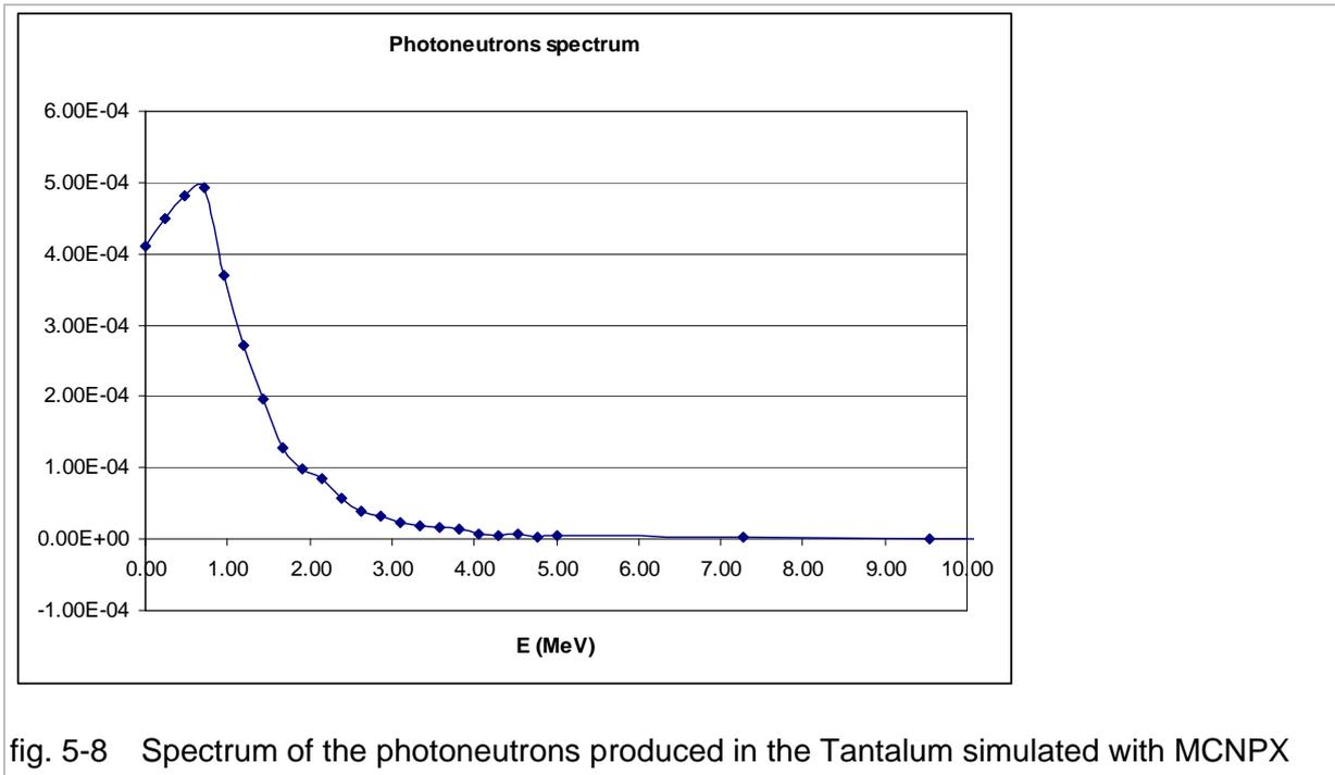
fig. 5-8 Spectrum of the photoneutrons produced in the Tantalum simulated with MCNPX
