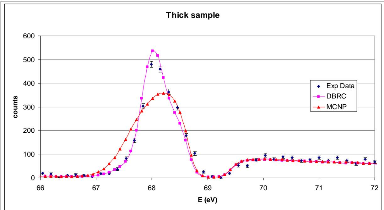
fig. 5-12 Thick sample, no moderator, 300 ns pulse width, 156° backscattering, 256 ns channel
