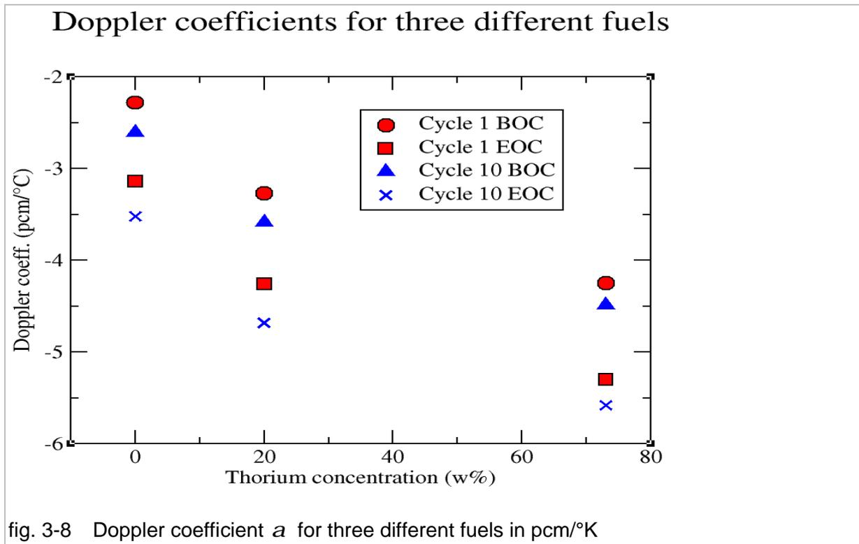
fig. 3-8 Doppler coefficient  $a$  for three different fuels in pcm/°K
