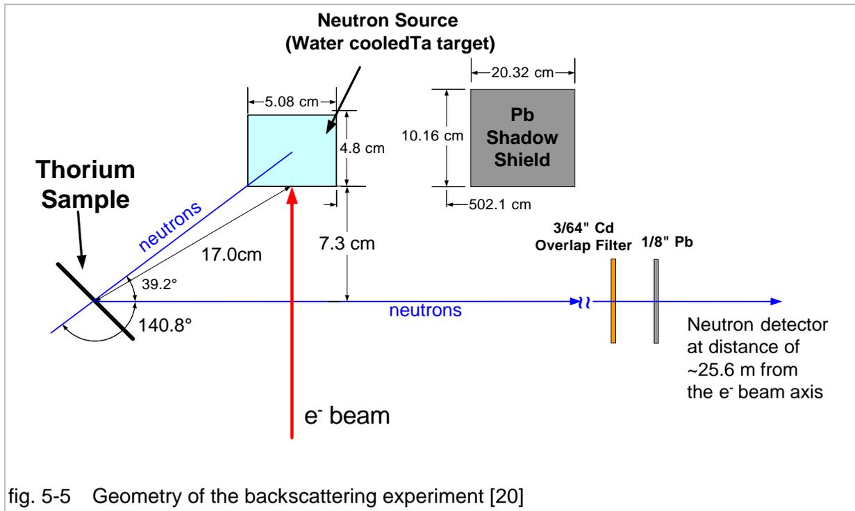
fig. 5-5 shows the geometry of the experiment as it was set up for the neutron resonance scattering kernel measurement on Th-232 and U-238. A summary of the results will be given in section 5.3.2.2.
