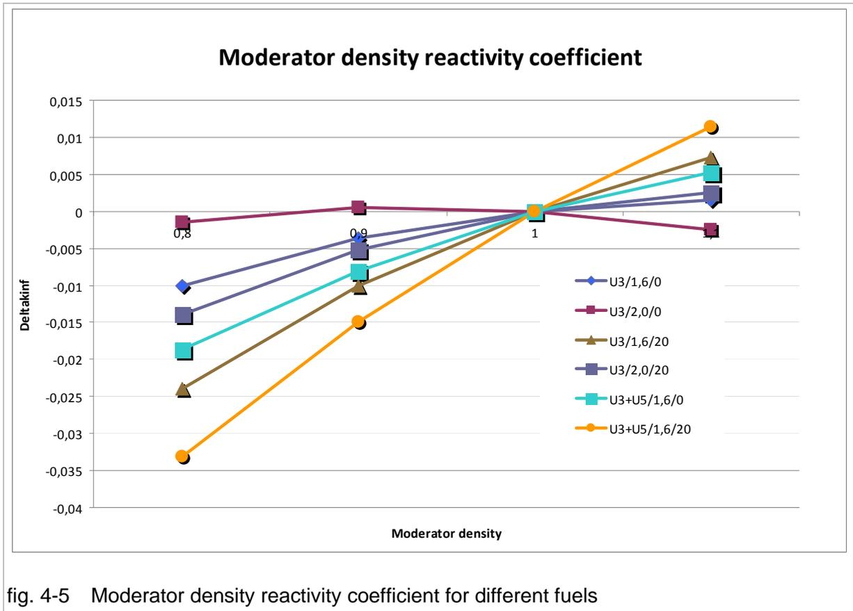
fig. 4-5 Moderator density reactivity coefficient for different fuels
