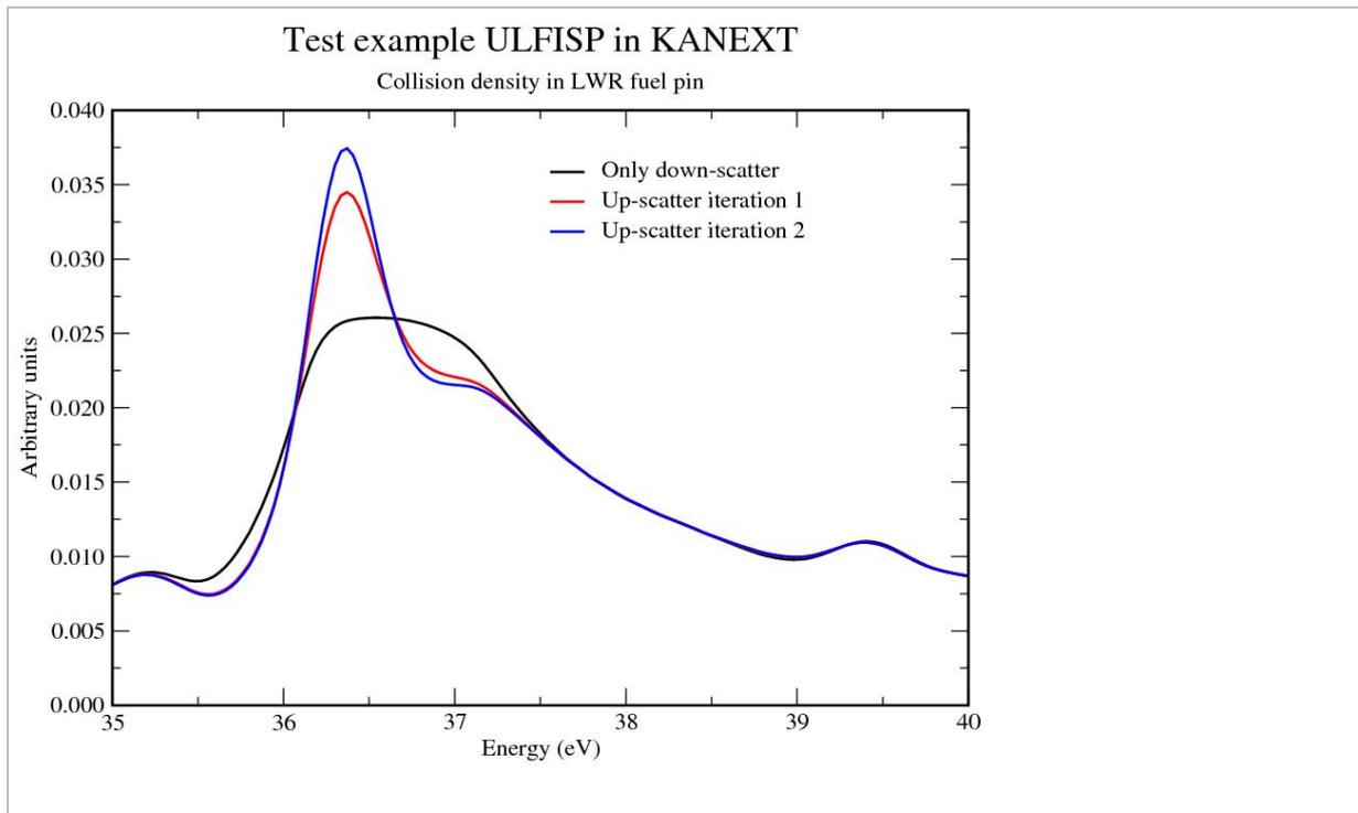
fig. 5-17 Collision densities in a LWR fuel pin containing U-238
