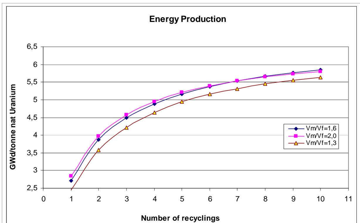
fig. 3-7 Energy production per unit of natural uranium consumed after each recycling for different moderation ratios of a fuel with 73% thorium
