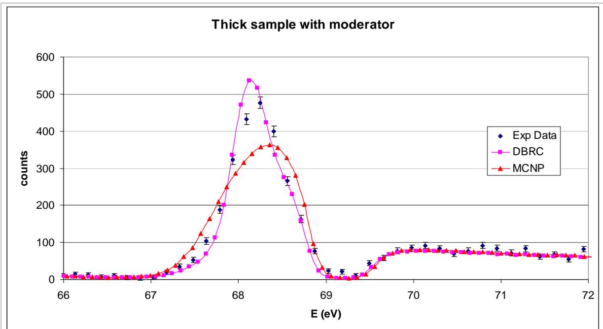
fig. 5-13 Thick sample, moderator, 300 ns pulse width, 156° backscattering, 256 ns channel
