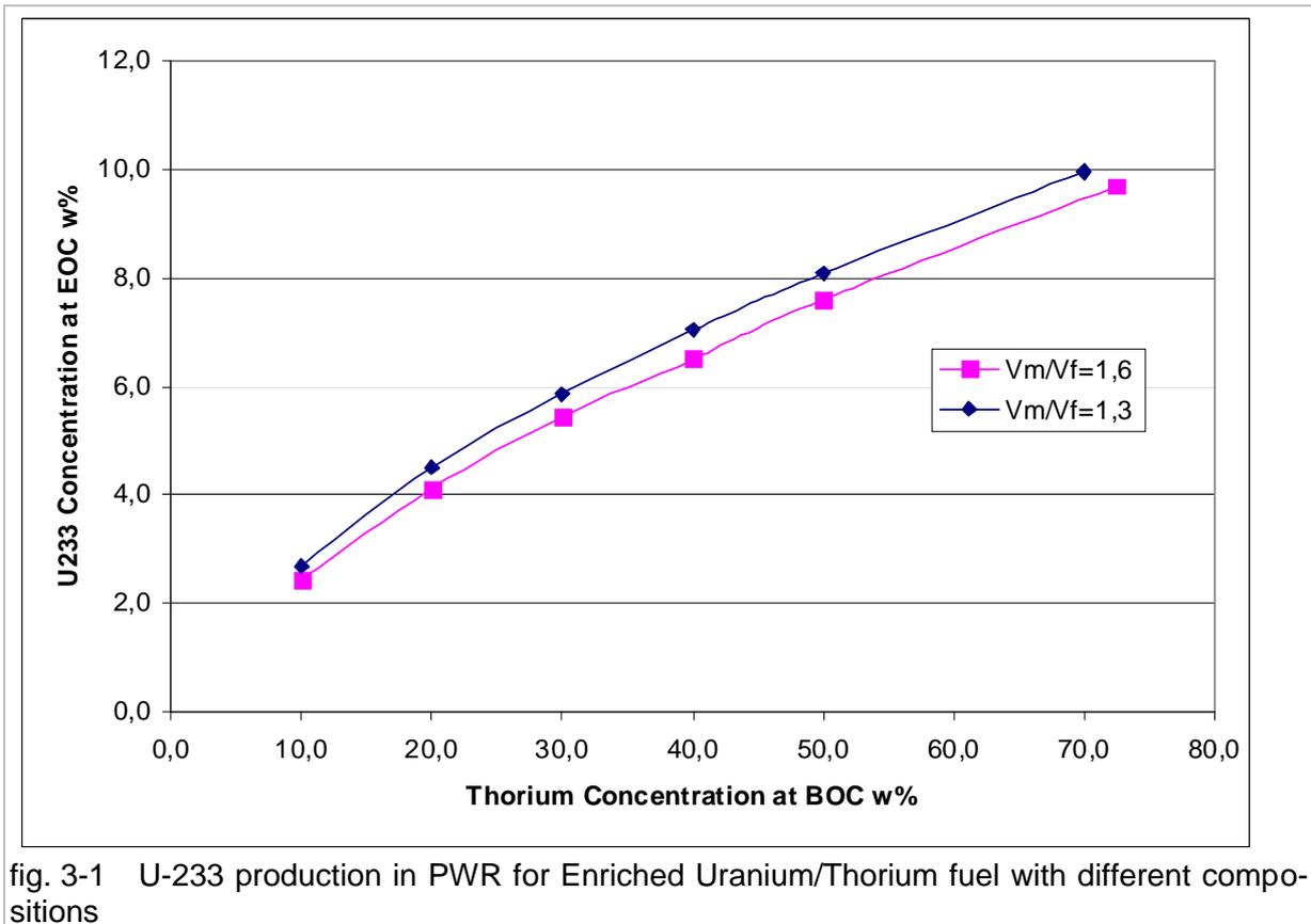
fig. 3-1 U-233 production in PWR for Enriched Uranium/Thorium fuel with different compositions
