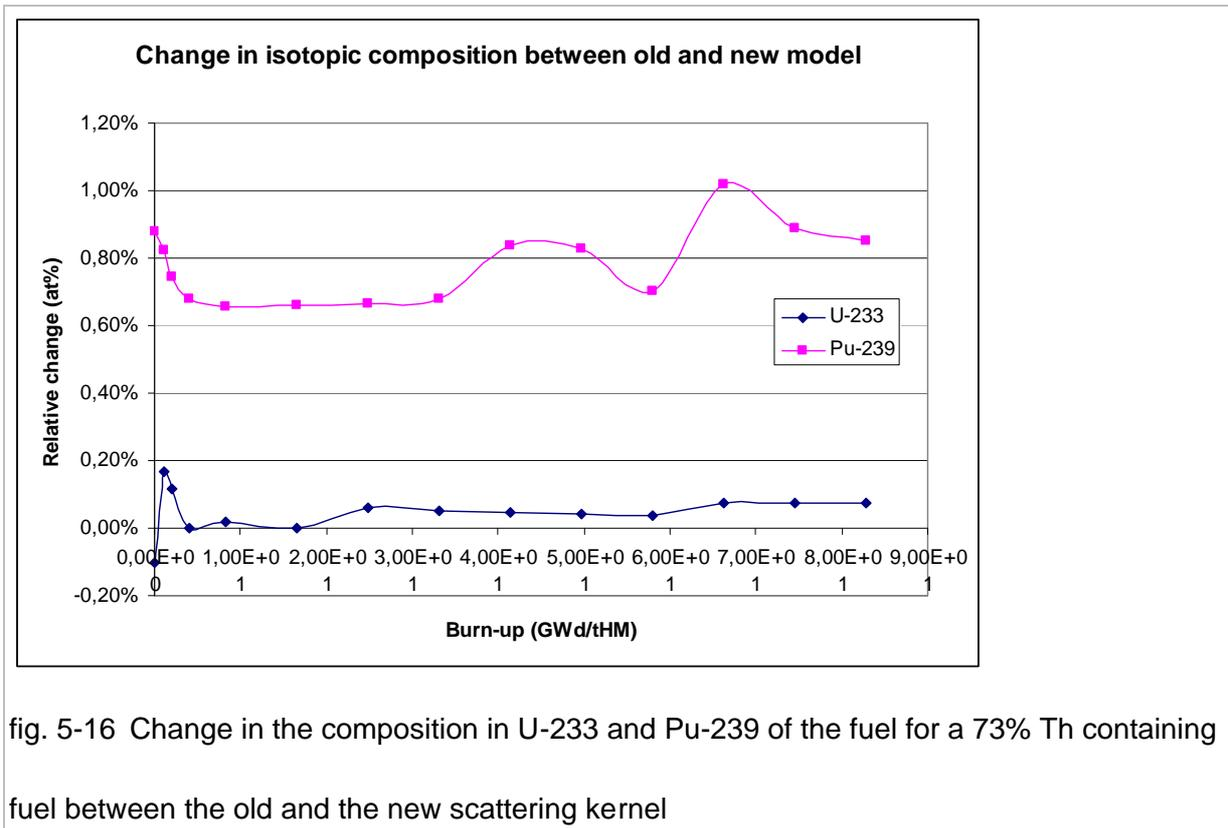
fig. 5-16 Change in the composition in U-233 and Pu-239 of the fuel for a 73% Th containing fuel between the old and the new scattering kernel
