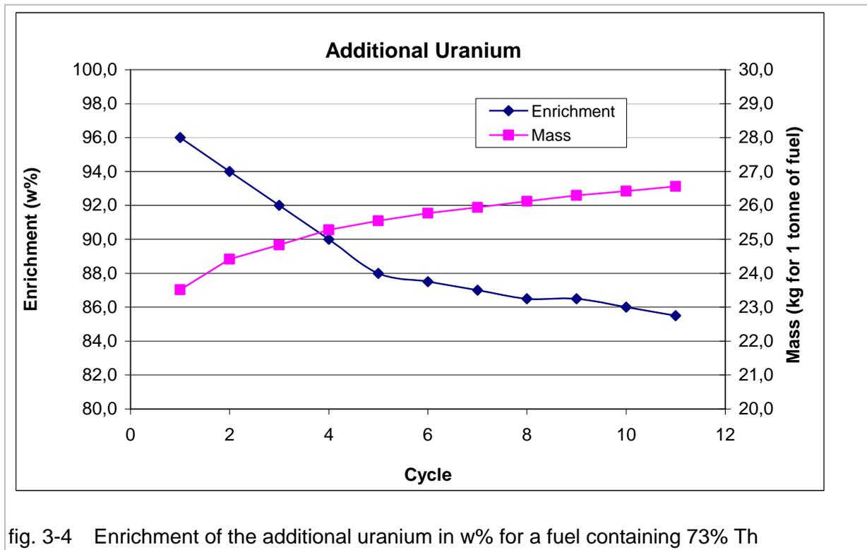
fig. 3-4 Enrichment of the additional uranium in w% for a fuel containing 73% Th
