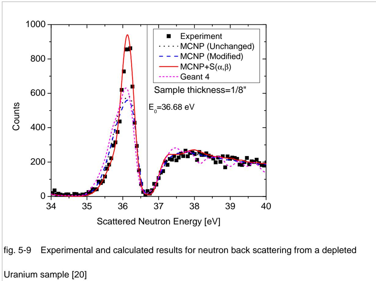
fig. 5-9 Experimental and calculated results for neutron back scattering from a depleted Uranium sample [20]
