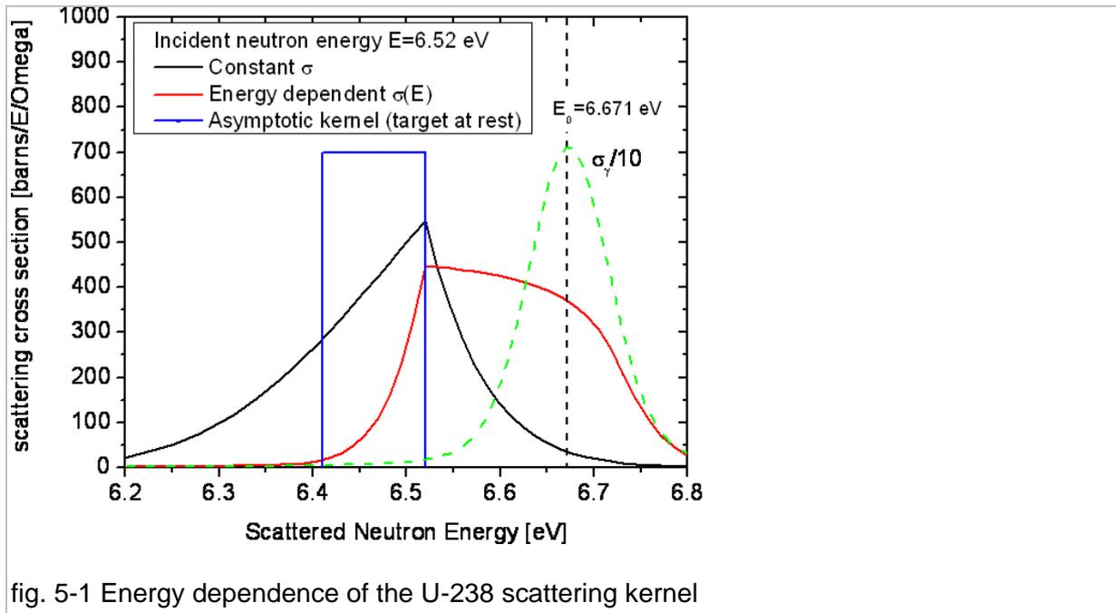
fig. 5-1 Energy dependence of the U-238 scattering kernel
