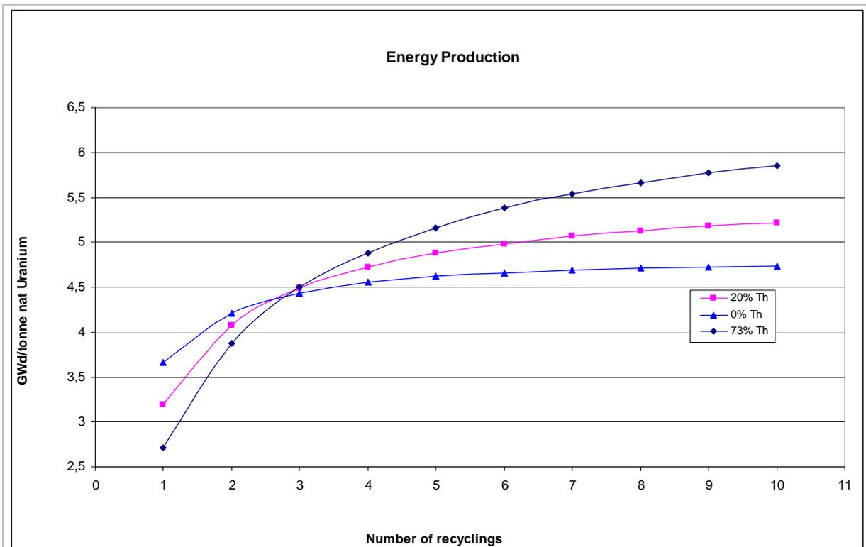
fig. 3-6 Energy production per unit of natural uranium consumed after each recycling for different thorium concentrations in the fuel
