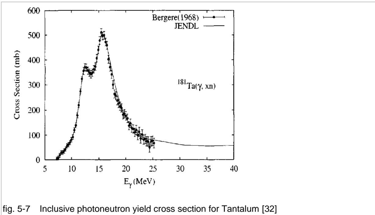
fig. 5-7 Inclusive photoneutron yield cross section for Tantalum [32]
