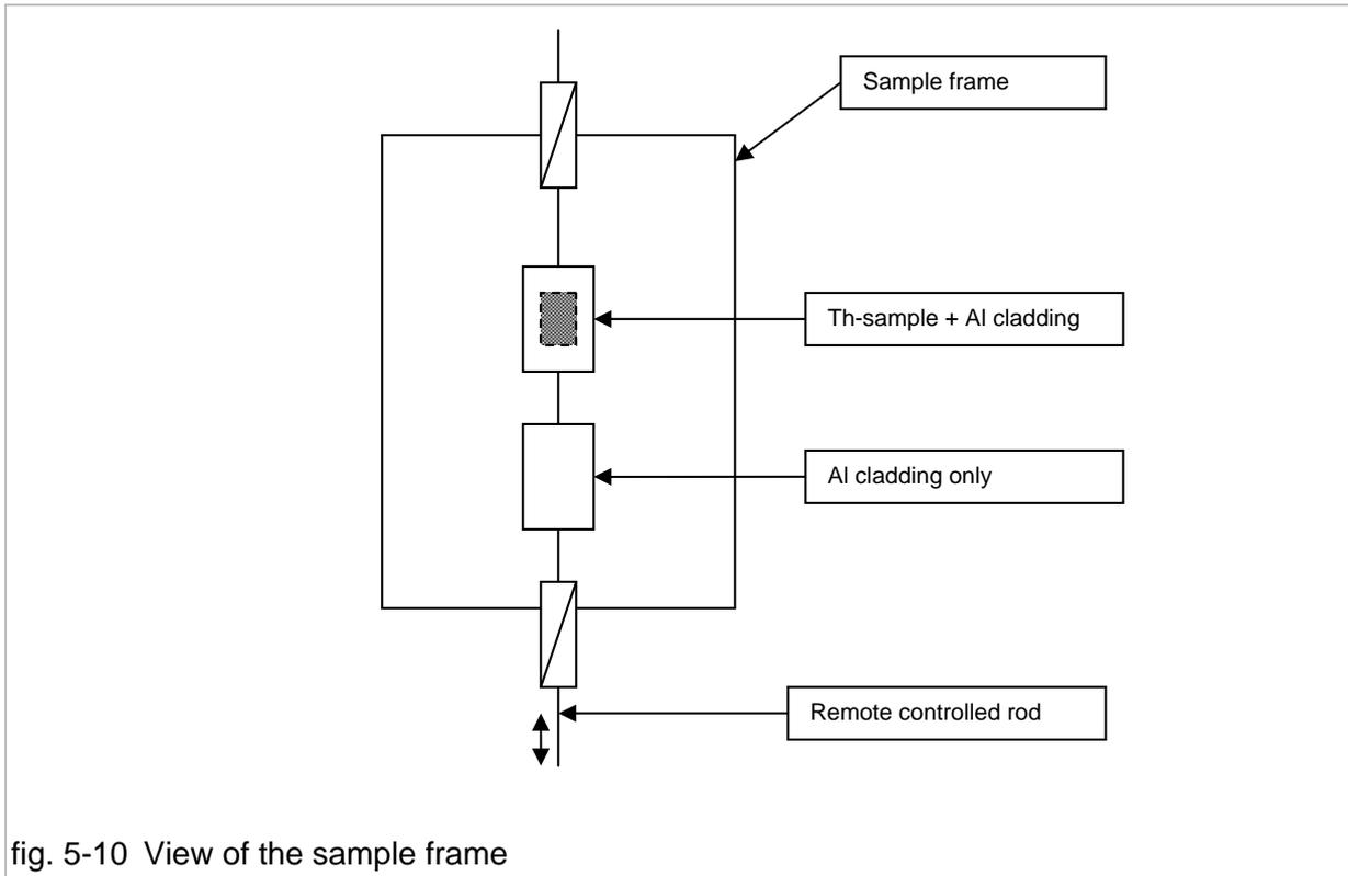
fig. 5-10 View of the sample frame
