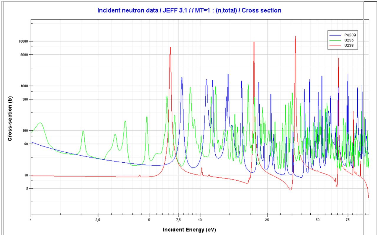
fig. B-1 Total cross section for U-238, U-235 and Pu-239
