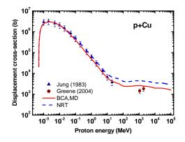
The total displacement cross-section for copper
