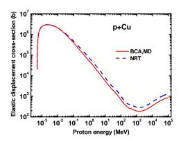
The elastic displacement cross-section for copper.
