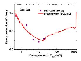
Example of combined BCA-MD calculations. The critical energy for Cu-ion is equal to 28.3 keV. The maximal  $T_{\text{dam}}(NRT)$  energy corresponds to the primary energy of Cu-ions 5 GeV.
