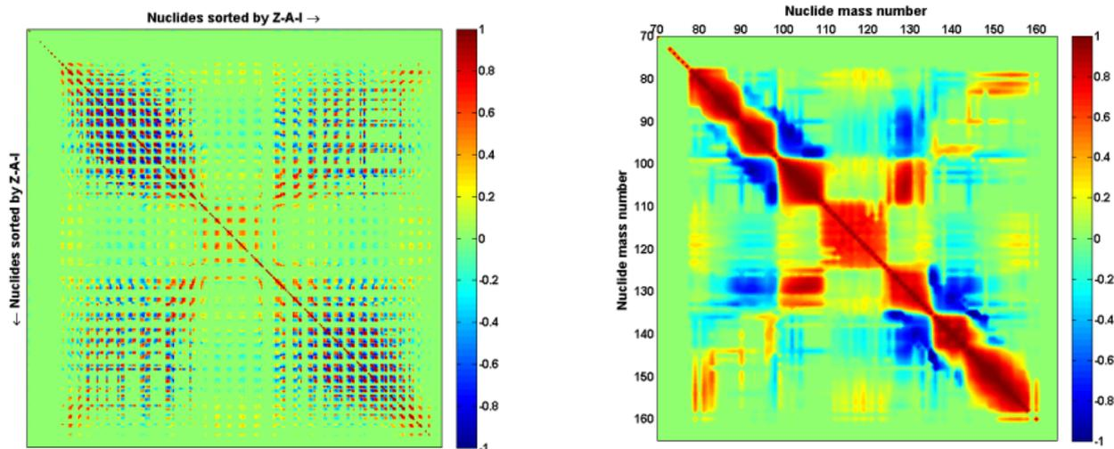
Figure 5: Plot of correlation matrix of fission product yields for  $^{235}\text{U}(n,F)$  induced by thermal neutrons. Yields given as a function of proton number, mass number and isomer (left) or only as a function of mass number (right). Visible anticorrelations originate from proton even-odd effect and competition between fission channels.
