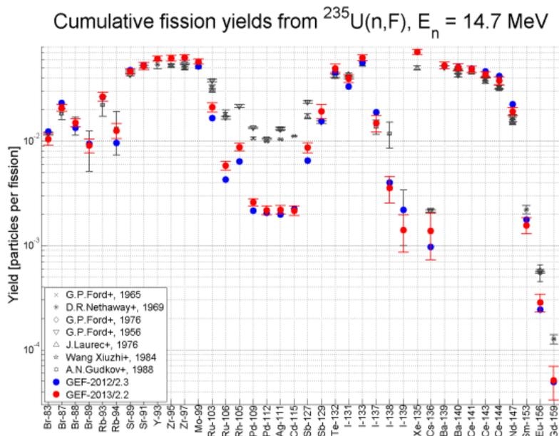
Figure 4: Cumulative fission product yields from  $^{235}\text{U}(n,F)$  induced by 14.7 MeV neutrons. Significant underestimation of FPY from the superlong mode around  $A = 115$ .
