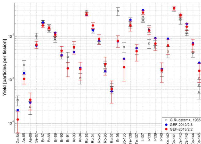
Figure 3: Cumulative fission product yields from  $^{235}\text{U}(n,F)$  induced by thermal neutrons, calculated from independent yields using ENDF/B-VII.1 decay data library. GEF results compared to EXFOR
