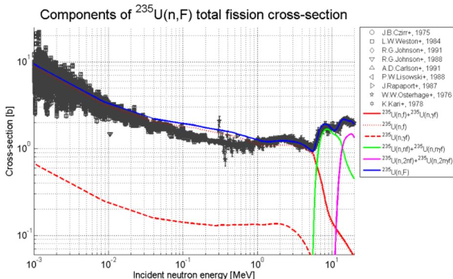
Figure 1: Below 5 MeV only first chance fission (solid red line), binary (n,f) reactions (dotted red line) dominating, pre-fission gamma emission (dashed red line) factor 10 smaller. Second (green line) and third chance fission (pink line) are very important above their respective thresholds.
